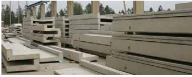
Figure 3: Precast concrete units.
