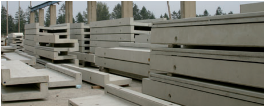
Fig. 1: Precast components made from lightweight aggregate concrete for the redevelopment of Wimbledon Centre Court, UK
