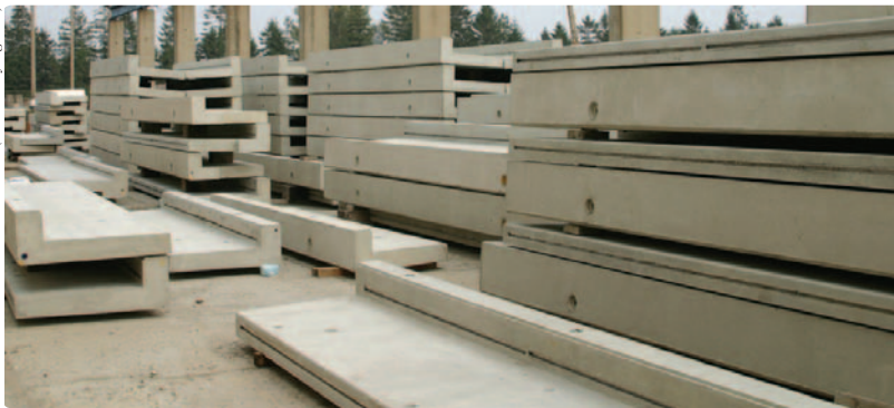
Figure 1: LWA precast components for Centre Court.
